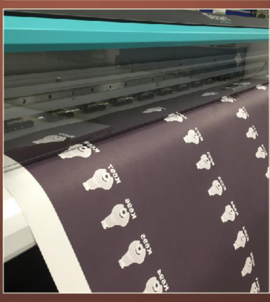
Dye sublimation printing uses heat to transfer ink from a paper backing onto specialty materials, including fabrics and ceramics. We handle 64-inch rolls with a full spectrum of CMYK ink. The most popular substrate is white polyester fabric, which is perfectly suited to mousepads, koozies, and other promotional textiles.
